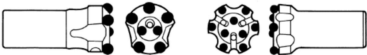
Figure 2. Typical 7- and 9-button bits used in hard rock tunnelling (Thuro 1997) and uses accordingly for the drilling investigations.
